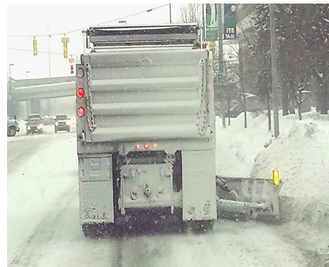
An example of a wing blade plow
